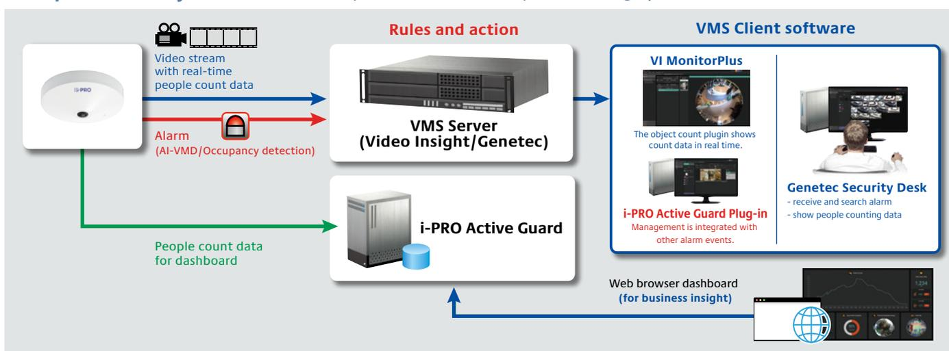
\*VMS Server and i-PRO Active Guard can be installed on the same server.
