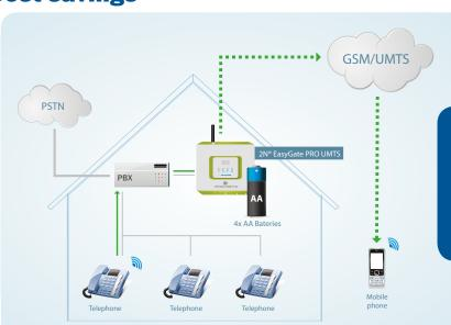
In this scenario, the firm connects the 2N® EasyGate PRO UMTS gateway via an analogue interface to its existing PBX. The exchange identifies a call to a mobile number and routes the call via the 2N® EasyGate PRO UMTS gateway. The gateway is accessible to all users of the exchange.
