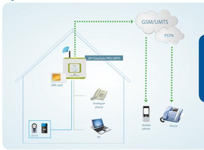
Connect an analogue telephone or PBX and start making calls. With a connected computer, you can also receive and send text messages or browse the internet. The 2N® EasyGate PRO UMTS can be used in areas where there is no landline, or the gateway can provide an alternative for users who no longer want to use a landline.
