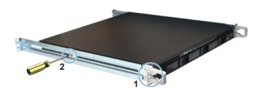
3 Fix the unit in the rack with the long screws that came with your rack. As the size of the screws varies according to rack models, check the package content that came with your rack.
